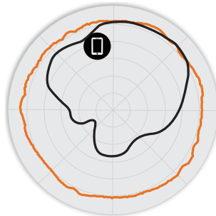
Figure 3. T301n 5GHz Azimuth Antenna Patterns
