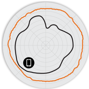
Figure 2. T300 2.4GHz Azimuth Antenna Patterns
