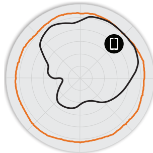
Figure 3. T300 5GHz Azimuth Antenna Patterns
