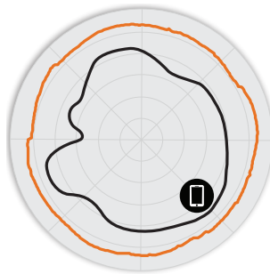
Figure 3. R720 5GHz Azimuth Antenna Patterns
