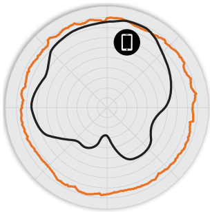
Figure 2. R720 2.4GHz Azimuth Antenna Patterns
