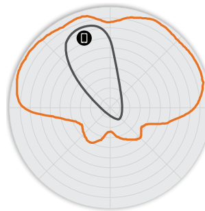
Figure 4. R720 2.4GHz Elevation Antenna Patterns
