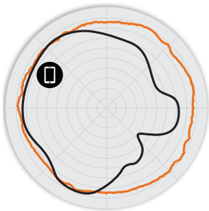
Figure 2. R310 2.4GHz Azimuth Antenna Patterns
