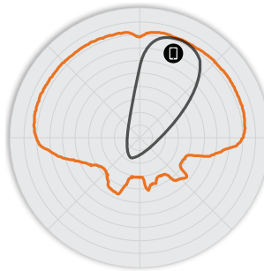
Figure 4. H510 2.4GHz Elevation Antenna Patterns
