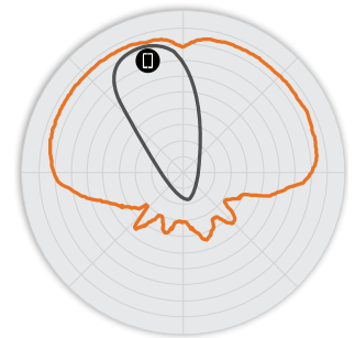
Figure 5. H510 5GHz Elevation Antenna Patterns
