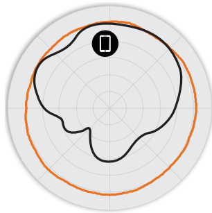
Figure 3. H510 5GHz Azimuth Antenna Patterns
